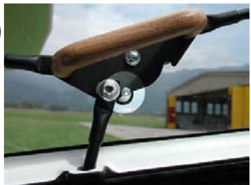
Correct - door secured
